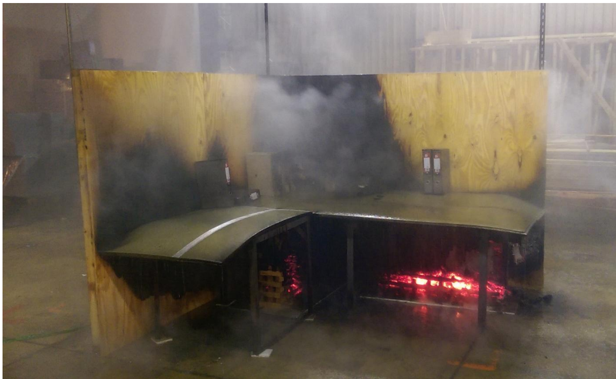
Figure 12 – Fire damage to the plywood walls, foam sheets and box files
