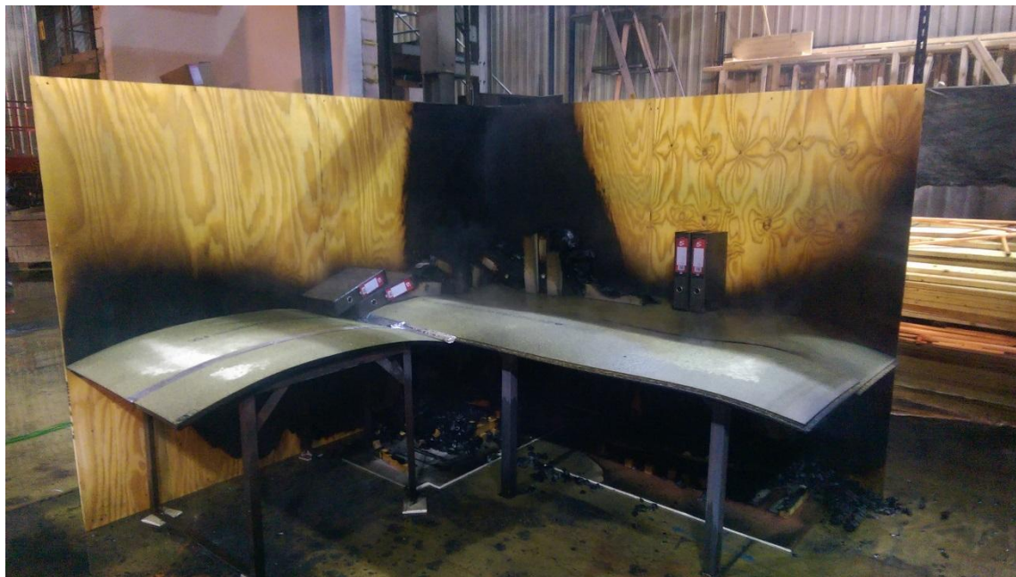
Figure 17 – Fire damage to the plywood walls, foam sheets and box files
