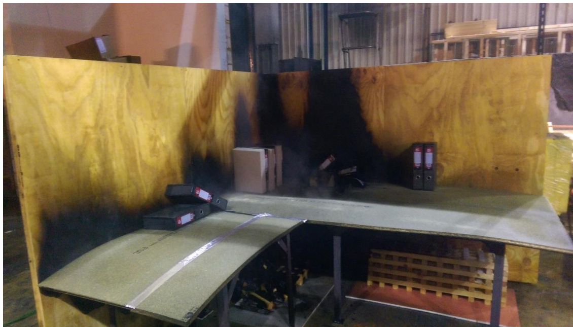
Figure 22 – Fire damage to the plywood walls, foam sheets and box files
